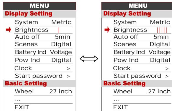
**8.3 Auto off** : Press UP/DOWN button to change the auto power off time, from 1 to 9 or OFF, the number represent time (minutes) to shutdown, default value is 5 minutes.
