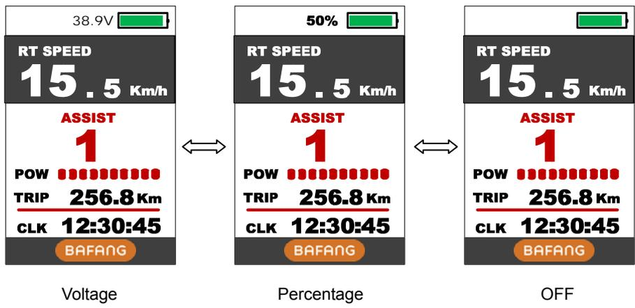
**8.6 Pow Ind :** Press UP/DOWN button to change the Power indicator, Analog / Digital/Current.
