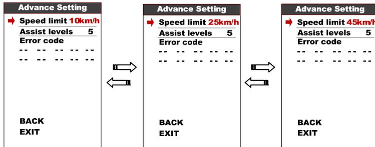
\*Speed limit and current limit are restricted by controller and motor.
