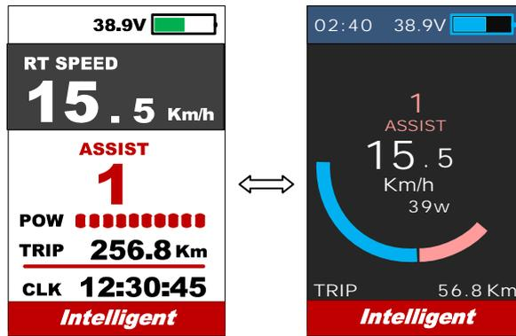
**8.5 Battery Ind** : Press UP/DOWN button to change the battery indicator, Voltage / Percentage / OFF.
